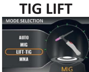
The TIG method is especially recommended for aesthetic and high-quality metal welding, without labour-intensive machining afterwards. However, this requires proper preparation and cleaning of the edges of both welded pieces. Mechanical properties of the additional material should be similar to those of the welded pieces. The shielding gas is pure argon, supplied in the amount according to the welding current settings.
